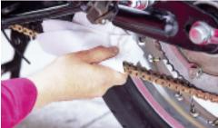
**4a.** After cleaning the chain, wipe the chain with a soft towel to remove any remaining dirt and chain cleaner. Rotate rear wheel by hand to clean the entire chain.
