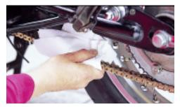
**8a.** After spraying on the chain lube, wipe the chain with a soft towel to remove excess chain lube. Rotate the rear wheel by hand and wipe the entire chain.
