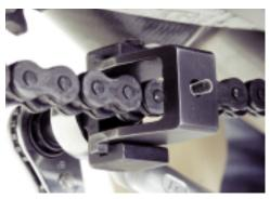
**5a.** Turn 19mm wrench clockwise on the tool's Hexagon bolt head to push the pin completely out.
