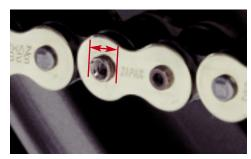
**16a.** Example of proper flared pin head. If your pin heads are not flared to this extent, Realign chain tool and flare pin heads until they look like the above photo. If your pin heads have cracks or the connecting link is stiff when flexed, remove connecting link and install a new one.
